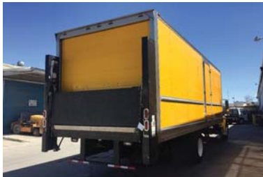
26FT DRY VAN W/ GATE 26' X 102" X 103" FRP VAN/SIDE DOOR MAXON 4400LB COLUMN LIFT STOCK#-65721 PRICE- $10,500
